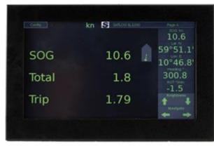
The <u>SKIPPER SATLOG SL1200</u> is a MED-B approved speed log measuring speed over ground (SOG) in three axis (Docking mode). It uses GPS and GLONASS systems in order to provide the longitudinal and fwd/aft transversal speed of the vessel relative to ground.
